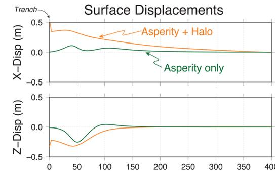
If we model only the effects of the asperity, the predicted deformation is incomplete (green). The halo of reduced slip also contributes to surface displacements (orange). An inversion of the full signal sees the halo as a zone of partial coupling. This coupling is due to proximity to the asperity, rather than being indicative of frictional characteristics at that point.
