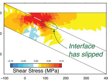
Modeled shear stress after freely sliding interface has slipped to resolve zero shear stress
