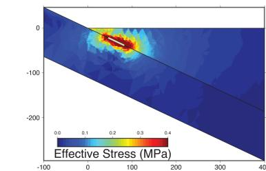
Effective stress is a measure of the amplitude of the stress tensor
